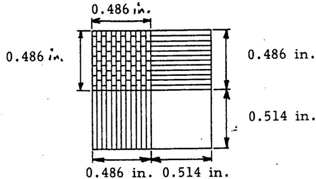
Figure 11. Threads are moved to the sides to illustrate area calculated by thread width times mesh number. Net free area is then calculated.
