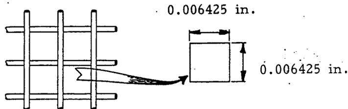
Figure 12. Net free area calculated from dimensions of individual openings.
