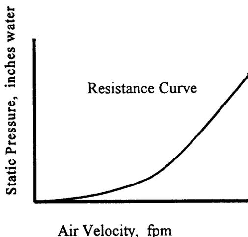
Figure 2. Curve showing pressure loss for air movement at different velocities through screening material.
