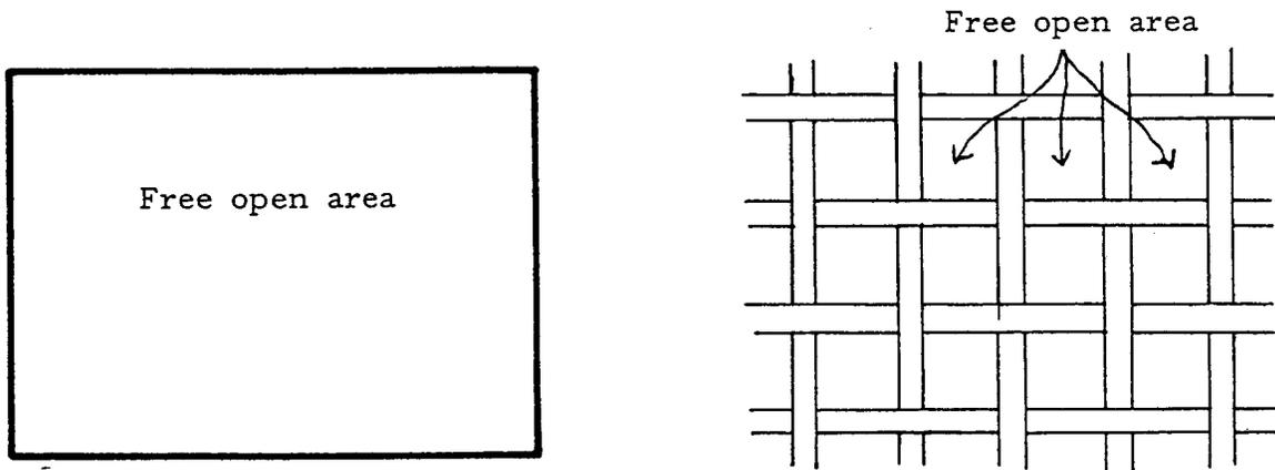
Figure 5. The free open area for air movement is reduced by the threads of the screening material.
