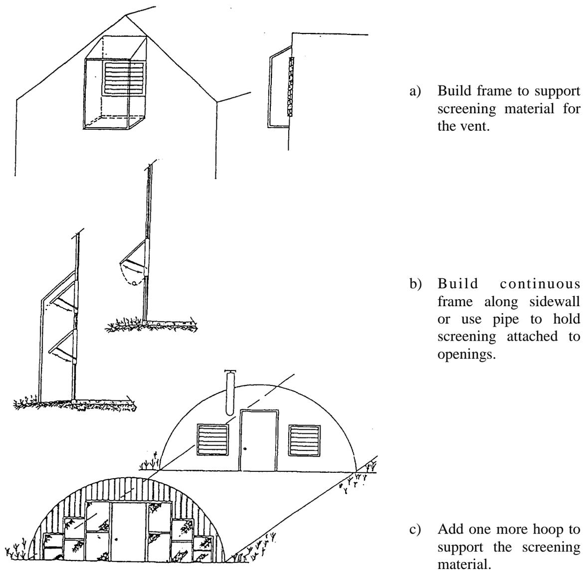
Figure 7. Illustrations of screening installations on greenhouses.
