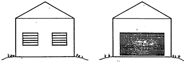
Figure 6. Screening material covers much greater area to allow same ventilation air flow.
