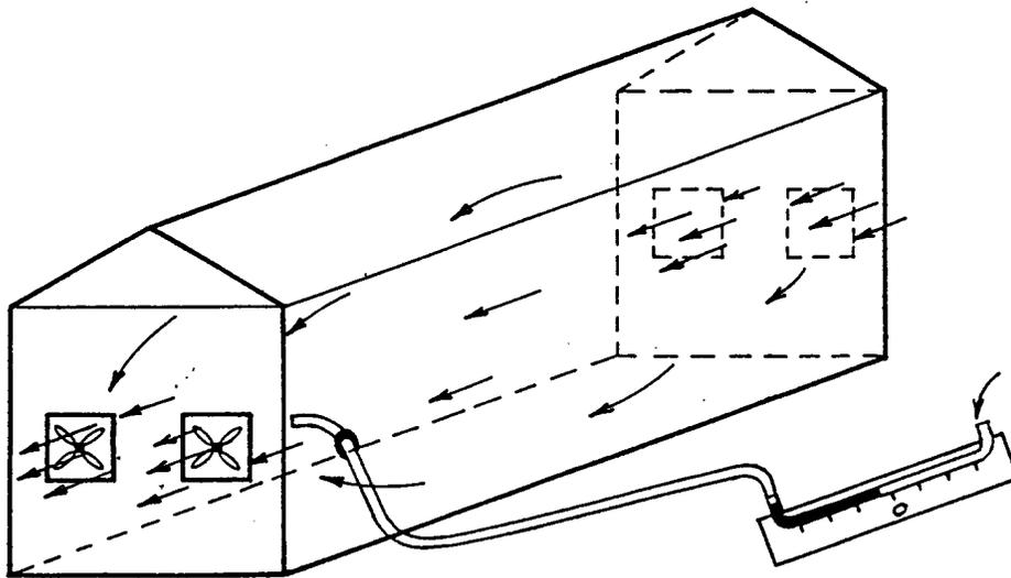
Figure 4. A manometer measures static pressure drop of air flow through greenhouse.
