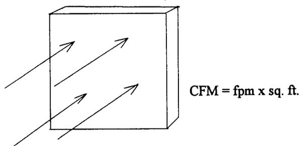
Figure 1. Ventilation air flow, CFM, is air velocity, fpm, times open area of louver, sq. ft.
